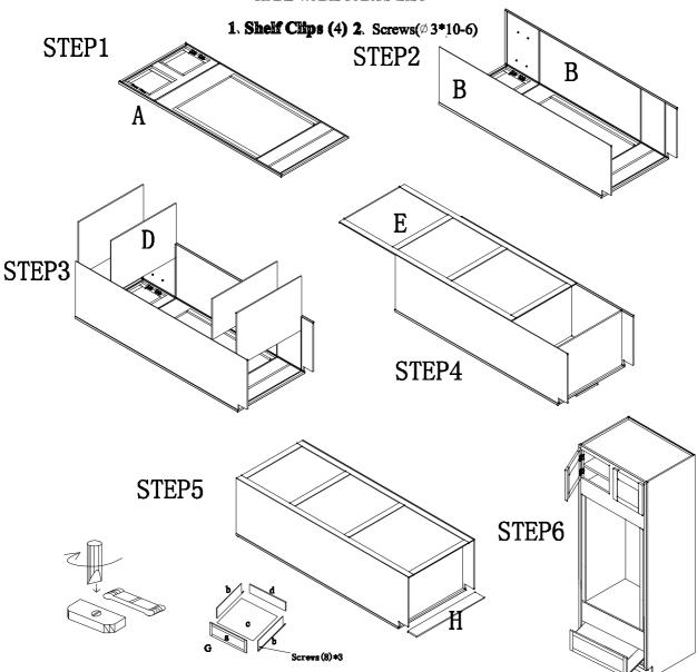
Your cabinet is complete. For installation, consult a professional contractor or building supplier for the proper installation method or materials to be used for your existing wall condition (e.g., wood, concrete, tile, etc.).
